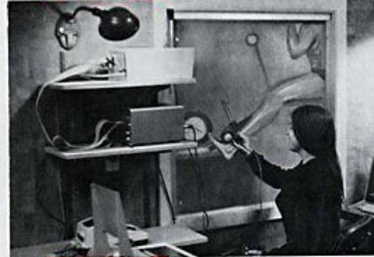
Special Tracing Equipment digitizes each joint movement for computer programming
